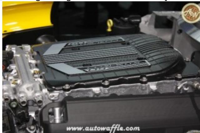
It's all thanks to this supercharged LT4, seen here on a cutaway model of the new Z06[/caption]
